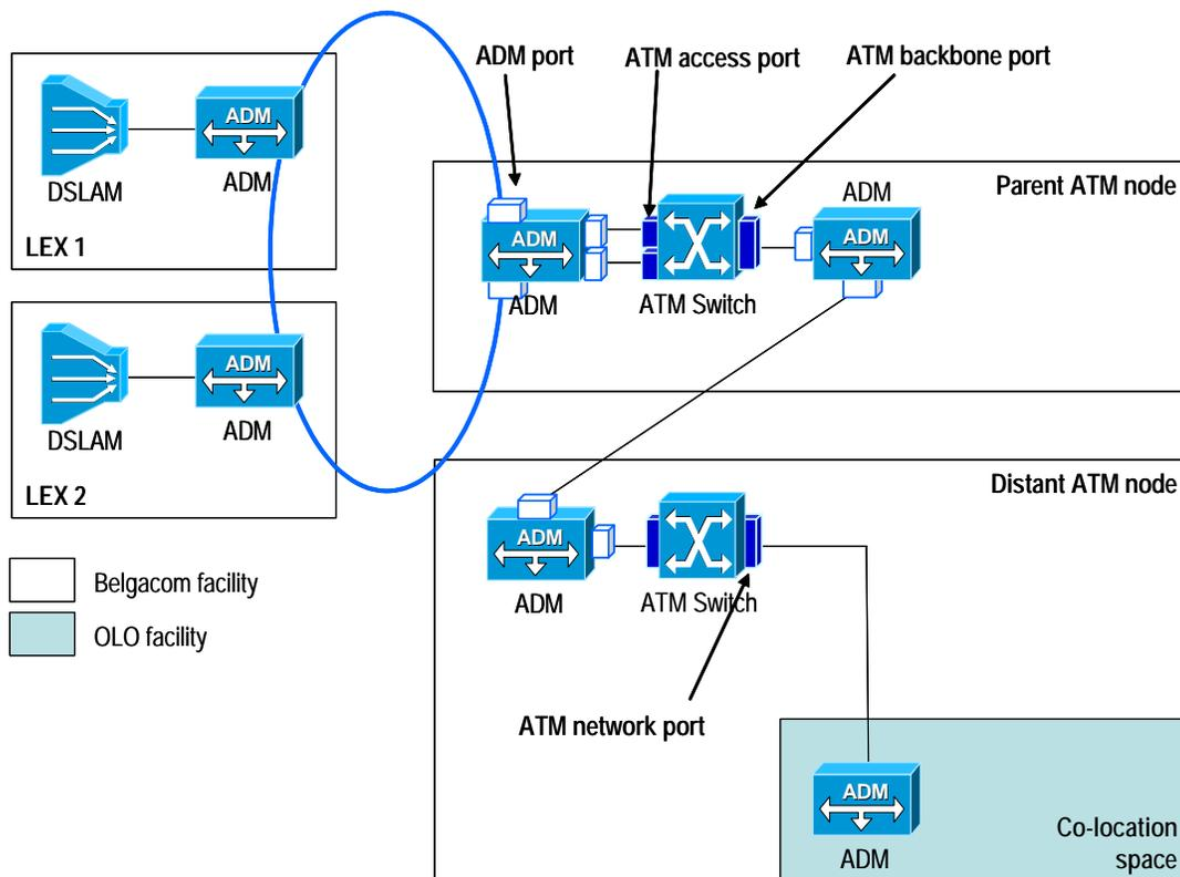
**Figure 5: survey of the components that are important in dimensioning the components in the situation where the OLO is not connected to each ATM node (non-local access scenario)**
