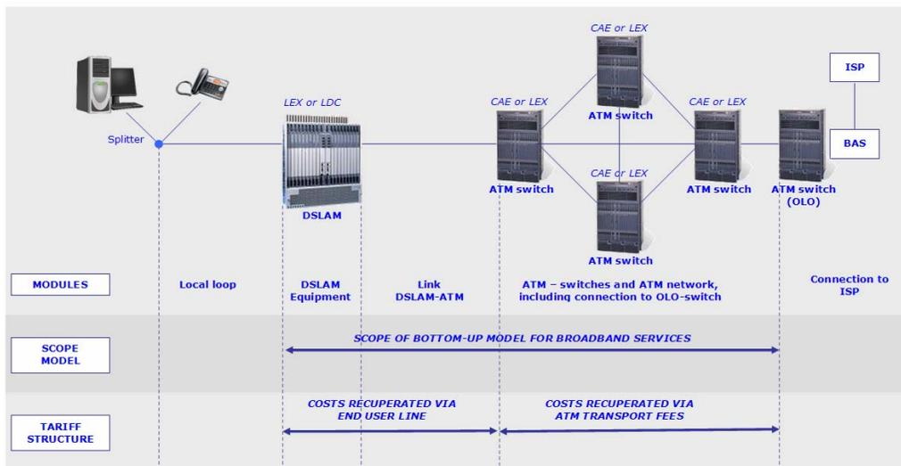
**Figure 1: Technical scope of the modeled network components for the provision of broadband services**
