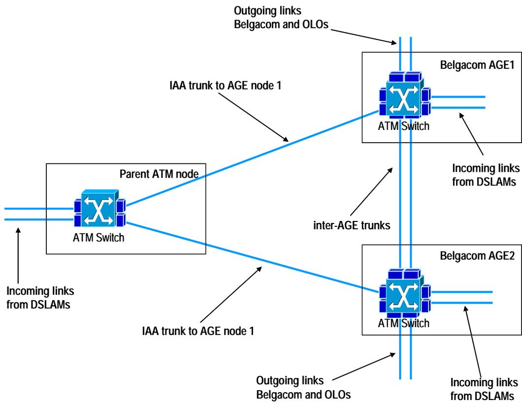
Figure 3: Diagram of the dimensioning in the situation where the OLO is not connected to each ATM node (non-local access scenario)
