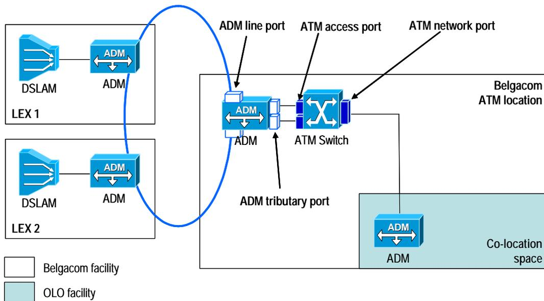
**Figure 4: survey of the components that are important in dimensioning the components in the situation where the OLO is connected to each ATM node (local access scenario)**
