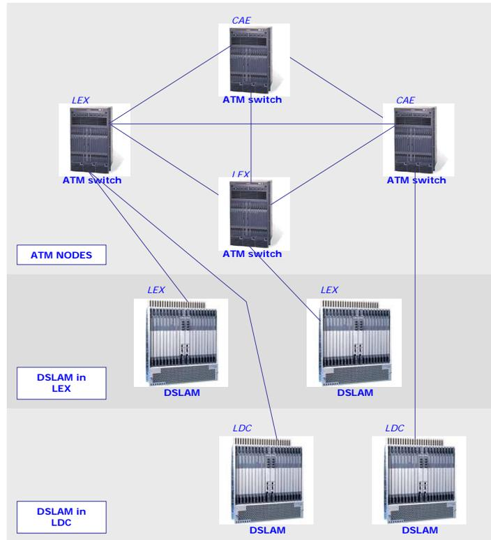
**Figure 3 Diagram of the topology of the specific network components in the BROBA bottom-up model**
